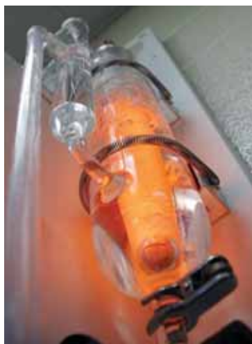
The treatment plant lab includes a Barnstead Mega Pure 3A water still (Thermo Fisher Scientific).
